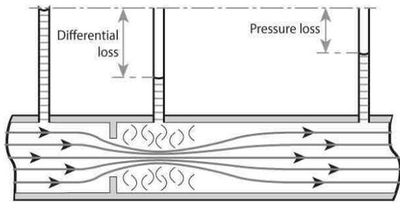
Figure 3-Pressure loss across the DP meter
