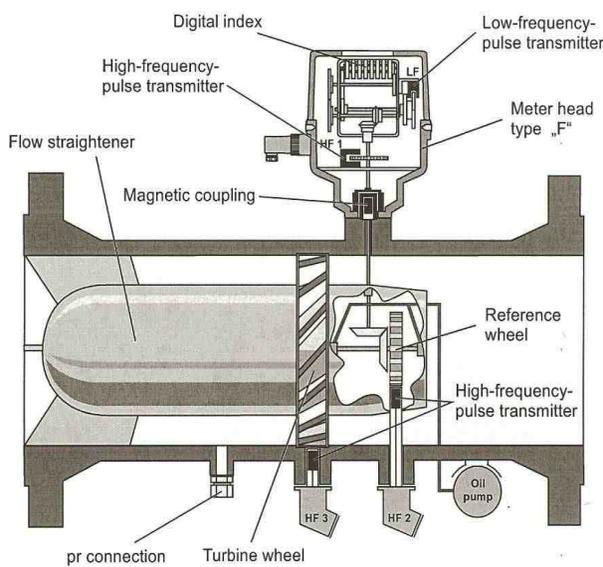
Figure 4-Cross section of a typical turbine meter
