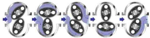
Figure 5-The oval gear positive displacement method
