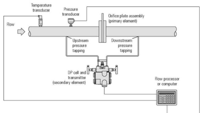
**Figure 2-A typical orifice plate steam flowmetering**
