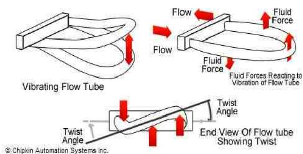
Figure 6-Coriolis principle of operation
