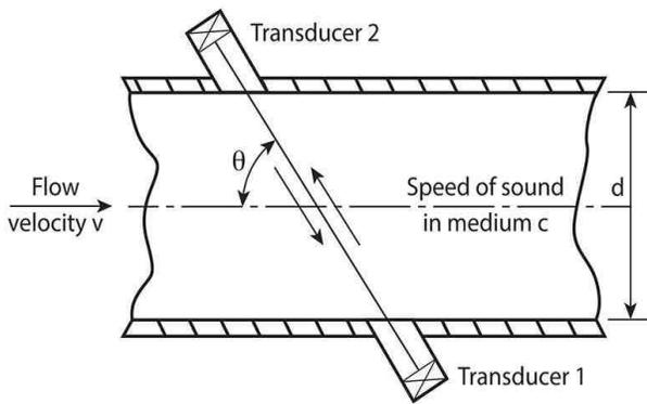
Figure 8-Ultrasonic meter schematic (single path)
