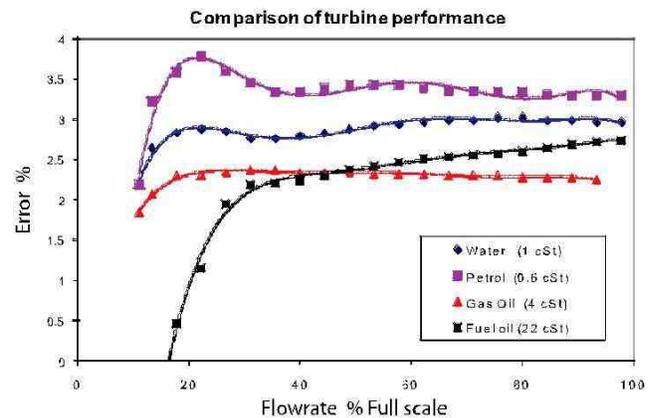
Figure 10. Turbine meter performance
