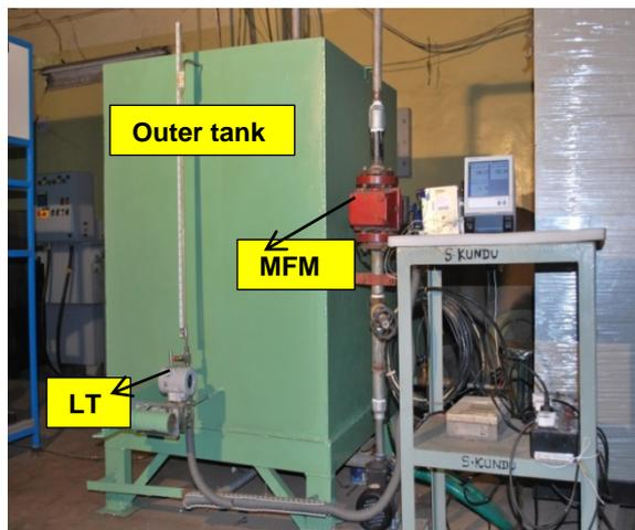
Figure 3: Passive Float Valve (PFV) experimental set up
