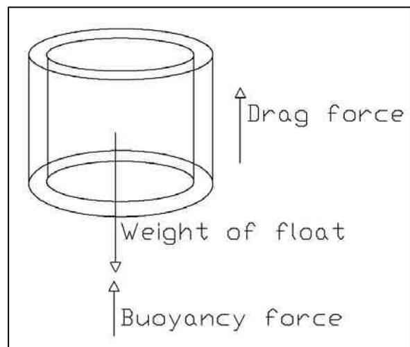
Figure 1. Force balance on the float
