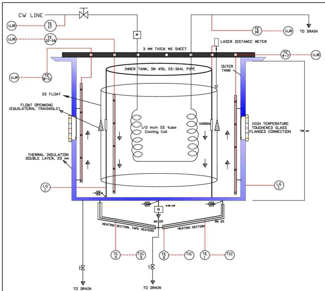
Figure 7: Natural circulation based Passive Float valve experimental set up
