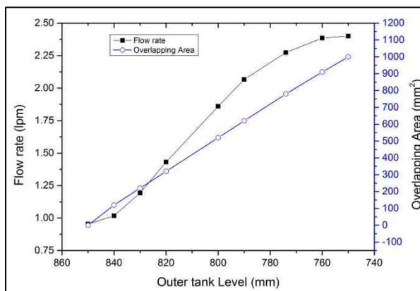
Figure 6: Float valve flow characteristics for 100 x 10 mm window
