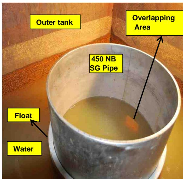
Figure 4: PFV floating around the outer periphery of the 450 NB pipe.
