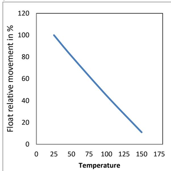
Figure 8: Float relative position (theoretical prediction) w.r.t, temperature of the primary coolant (Silicone oil).
