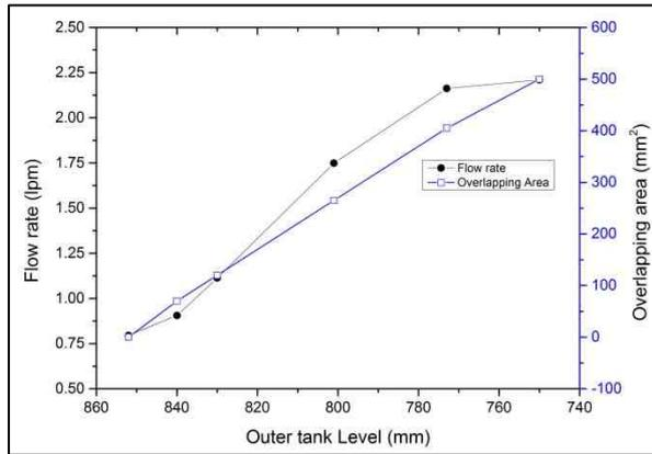
Figure 5: Float valve flow characteristics for 100 x 5 mm window
