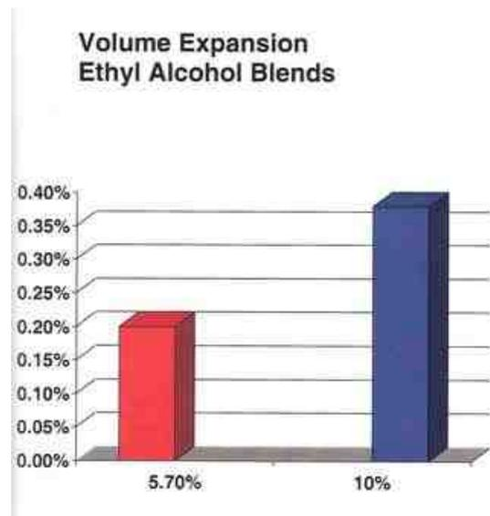
Figure 2.0 Volume expansion of ethanol in gasoline
