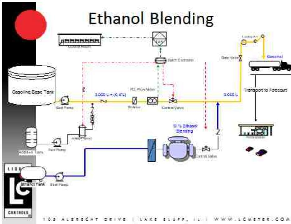
Fig 6.0 Ethanol blending process
