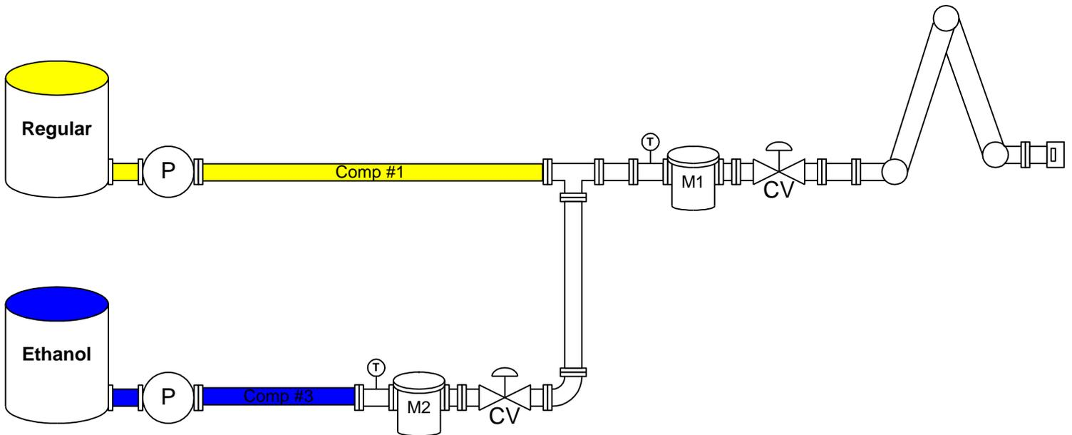
Fig 7.0 Side –stream blending schematic
