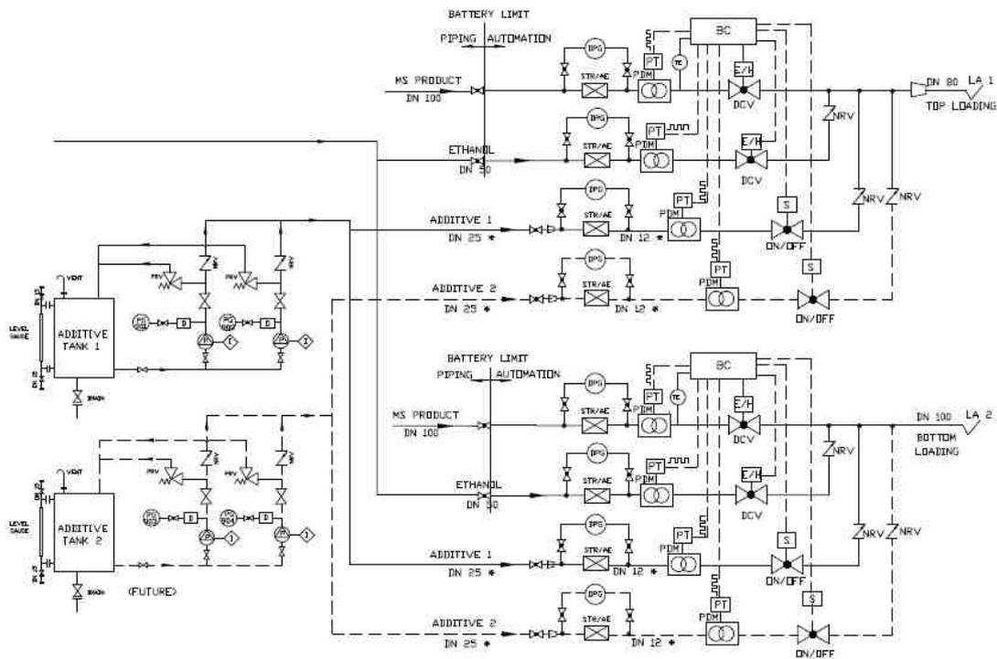
Fig 3.0 Typical P&ID of the loading of gasohol with Ratio blending
