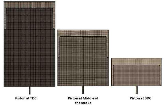
3: Section view of unstructured polyhedral mesh for different piston position
