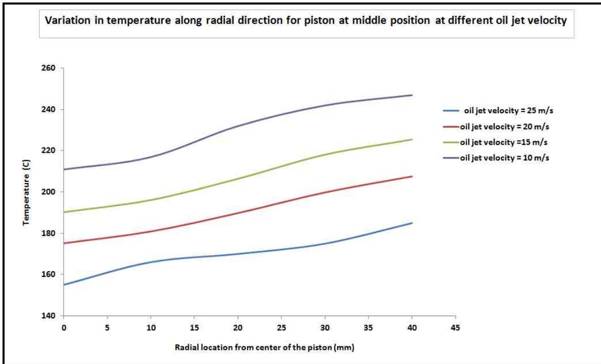
Fig.8 Variation in temperature along radial direction for different plots for piston at different position
