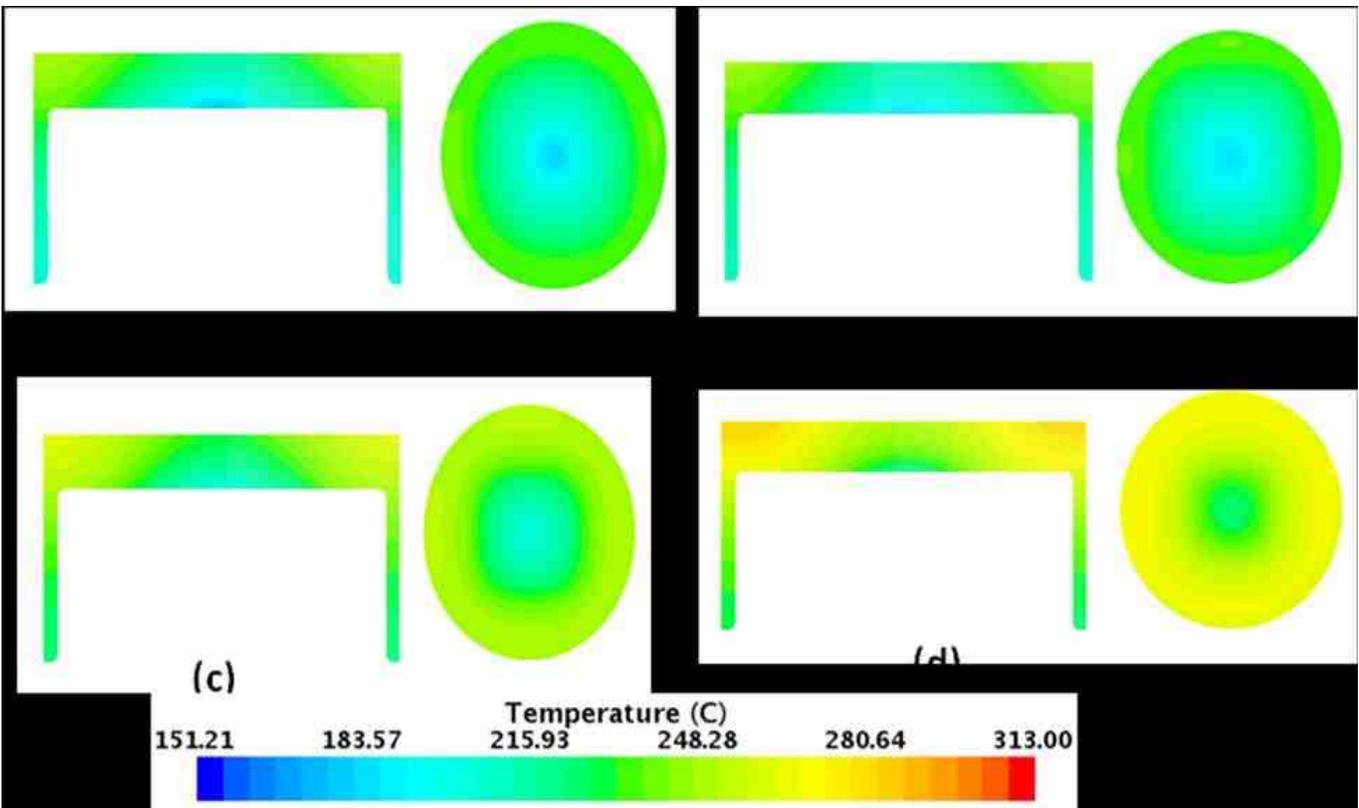
Fig.4 Temperature contour plot of piston at TDC with different oil jet velocity (a) 25 m/s (b) 20 m/s (c) 15 m/s (d) 10 m/s
