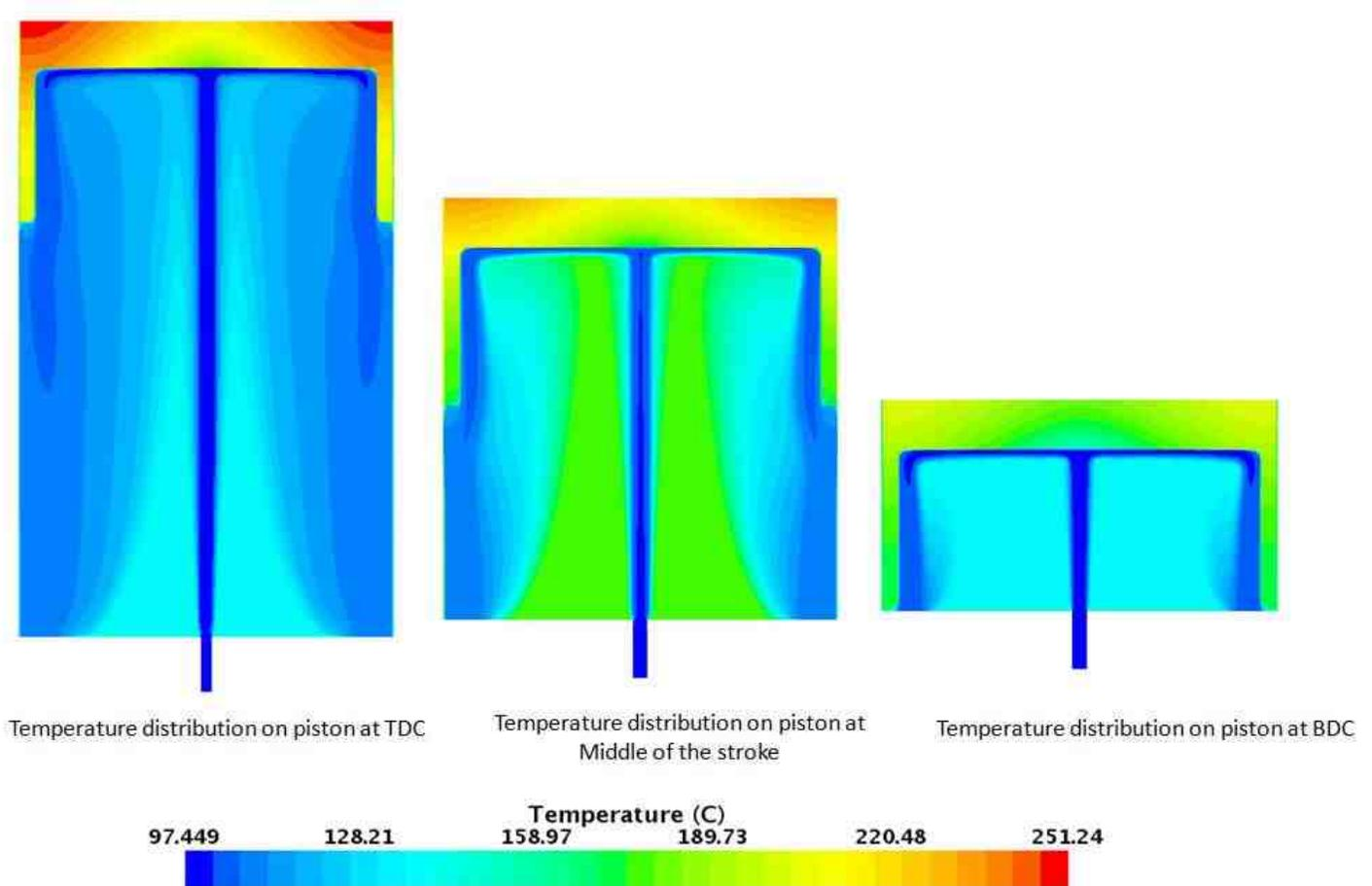
Fig .7 Temperature contour plots for piston at different position
