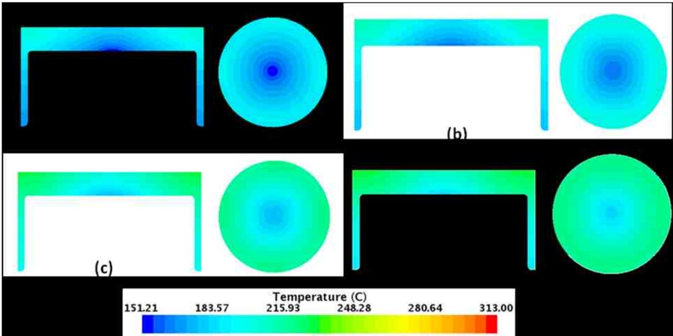
Fig.6 Temperature contour plot of piston at BDC with different oil jet velocity (a) 25 m/s (b) 20 m/s (c) 15 m/s (d) 10 m/s
