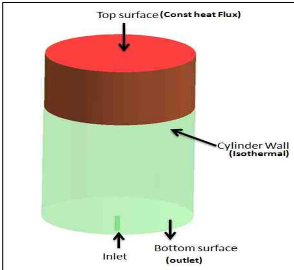
Figure: 2.1 Computational domain of single jet impingement
