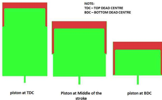
Figure: 2.2 Section view of piston position in the domain.
