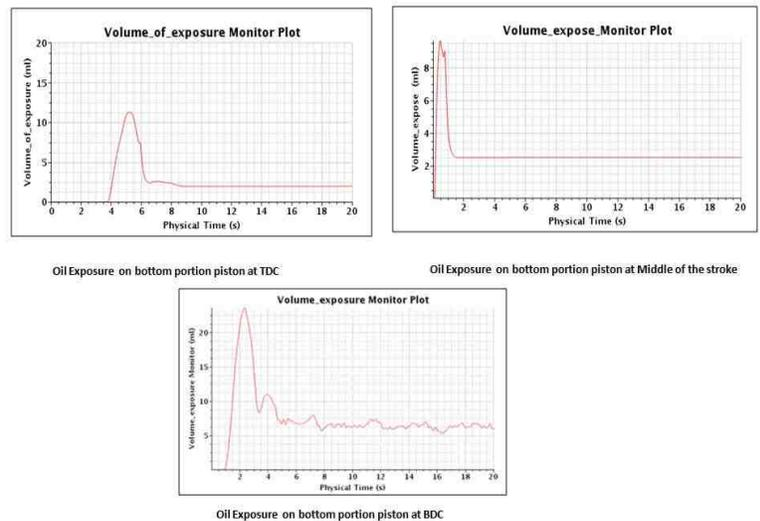
Fig.9 Volume of exposure of oil monitor plot for piston at different position
