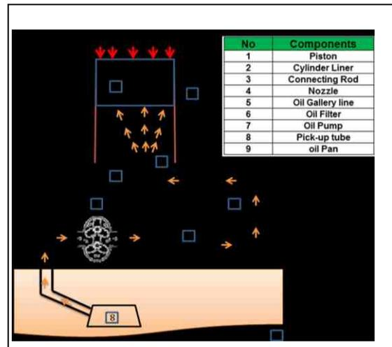
Figure: 1 Schematic sketch piston cooling using oil jet
