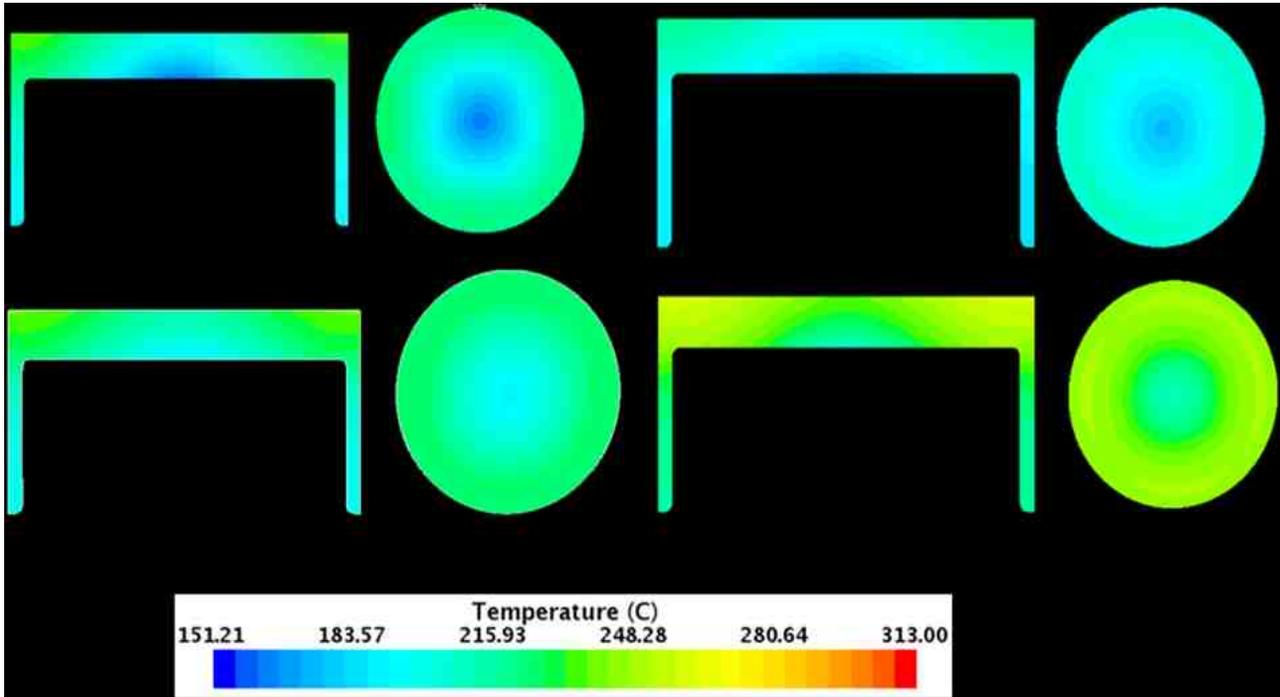
Fig.5 Temperature contour plot of piston at Middle of the stroke with different oil jet velocity (a) 25 m/s (b) 20 m/s (c) 15 m/s (d) 10 m/s
