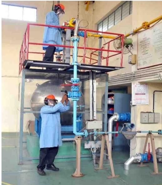
*Plate 3 Primary Standard Gravimetric System*
