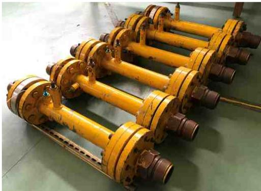
Plate 1 Critical Flow Venturi Nozzles
