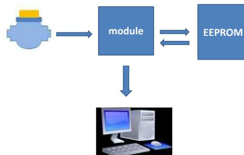
**Figure 1:** Data flow path in prototype system
