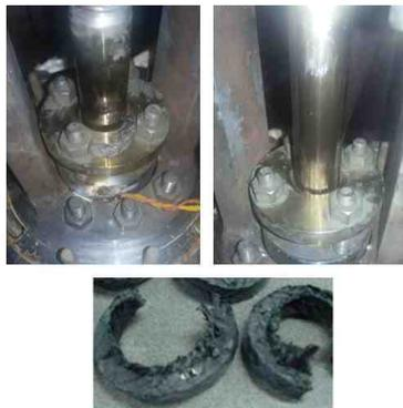
**Fig. 11 Damaged Graphite Packing**
