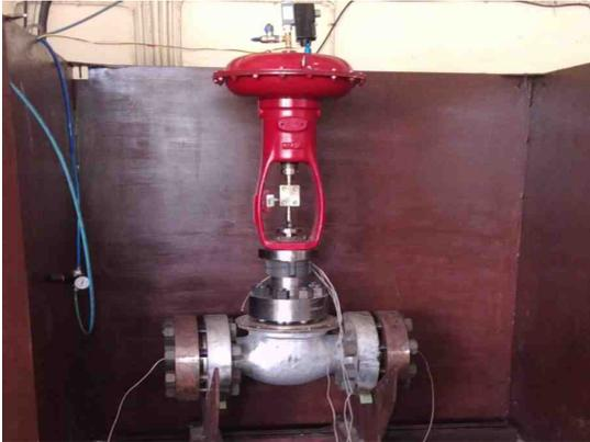
Fig. 6a Valve under Test
